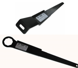
OCTAGONAL OR 2 EARED STEEL SPINNER REMOVERS
